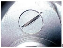
The first challenge is removing the slotted plug from the flywheel. Removing this plug gives you access to the sludge tube. The plug should not have been Loctited and should only be prevented from unscrewing by the center punch on the face of the flywheel.
