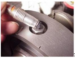
I use a Tempastick to determine when I reach the temperature I am looking for. I try to constrain the heating to the head of the bolt. If I am having trouble getting the Loctite to release I apply localized heat to the bolt retaining area at the crankshaft. Lacking a Tempastick one can use a drop of water which will sizzle when the temperature reaches 200 – 212 F.
