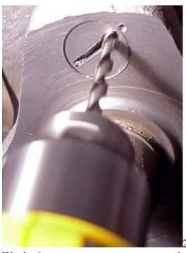
We don't want to put any more stress risers on the face of the flywheel, so we start by drilling straight into the face of the plug. What we want to do is only remove the flywheel metal that is pushed against the plug.
