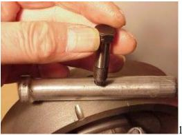
When you offer the new or cleaned tube to the flywheel, be sure to locate it so as the "tit" on the flywheel bolt can enter the larger of the three holes. Look down the flywheel hole to be sure the hole is properly aligned before offering the flywheel bolt.
