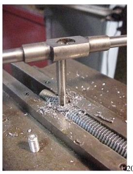
The 1/4" allen grub screw is in fore ground while the threaded rod is being tapped 1/4" x 20.
