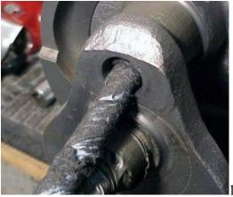
Use a screw driver, gun brushes and some spray brake cleaner (CRC Brakleen) and scrape and brush until the tube starts to get clean. Then wrap a paper shop rag around a medium sized screw driver and twist it into the hole. More spray cleaner and a half dozen, or more rags, clean the hole until you think it is spotless, and as my mentor always said, "Then clean for another ten minutes."
