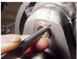
Hex driver flywheel plugs are the way to go (Use a relaible dealer as there are some oversize ones being sold). To have as few stress risers as possible I like to re-punch the face of the plug, instead of the flywheel, into the area that was originally punched. his leaves the crankshaft with only the original stress riser from the original center punching.
