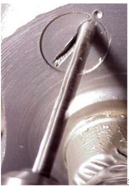
We started the drill a little bit back from the edge of the face of the plug and now we need to work the drill bit toward the edge and the center punch divot. Slowly tip the drill aiming it toward the edge and let it start cutting away the folded metal. To free the plug you will have to remove a little bit of the flywheel in the area of the divot, but be careful. Remove as little as possible.
