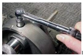
The flywheel bolt must be tightened to 33 foot pounds. Resist the temptation to believe that the Triumph engineers didn't know what they were doing and over tighten this bolt. It would be a real pain if the bolt broke as you tighten it. Worse, if it broke later at speed.
