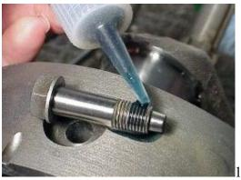
A few drops of blue Locite and the flywheel bolt is ready to be installed (If you are racing use Locite 270, but be sure you use enough heat to release it when doing future service.
