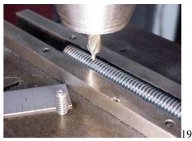
Using a short length of 1/2" threaded rod available in most big box stores for a few dollars and a 1/4" x 1/2" x 20tpi allen head grub screw you first drill and tap the rod 1/4" x 20.
