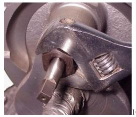
Tighten the nut against the face of the flywheel to withdraw the tube.
