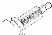
A waterproof plug-cover prevents the danger of plug failures caused by the accumulation of dirt on the insulator and the leakage of H.T. current across the dirty surface.
