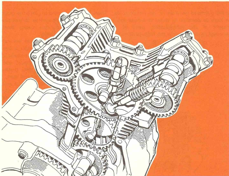
Intricate valve gear of the Overhead Cam 4 valve Honda CR110
