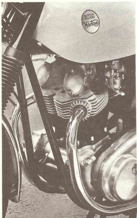
Norton 750cc Atlas engine—one of the biggest and most powerful in production
