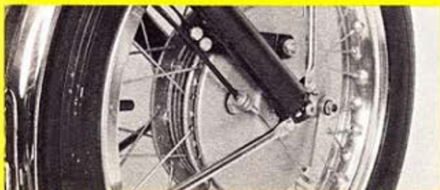
Powerful 190mm racing front brake, alloy racing wheel rims.
