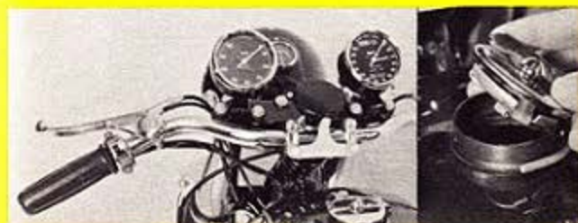
New 1963 type rubber insulated mounts for tachometer and speedometer. Inset: Quick-fill tank cap.
