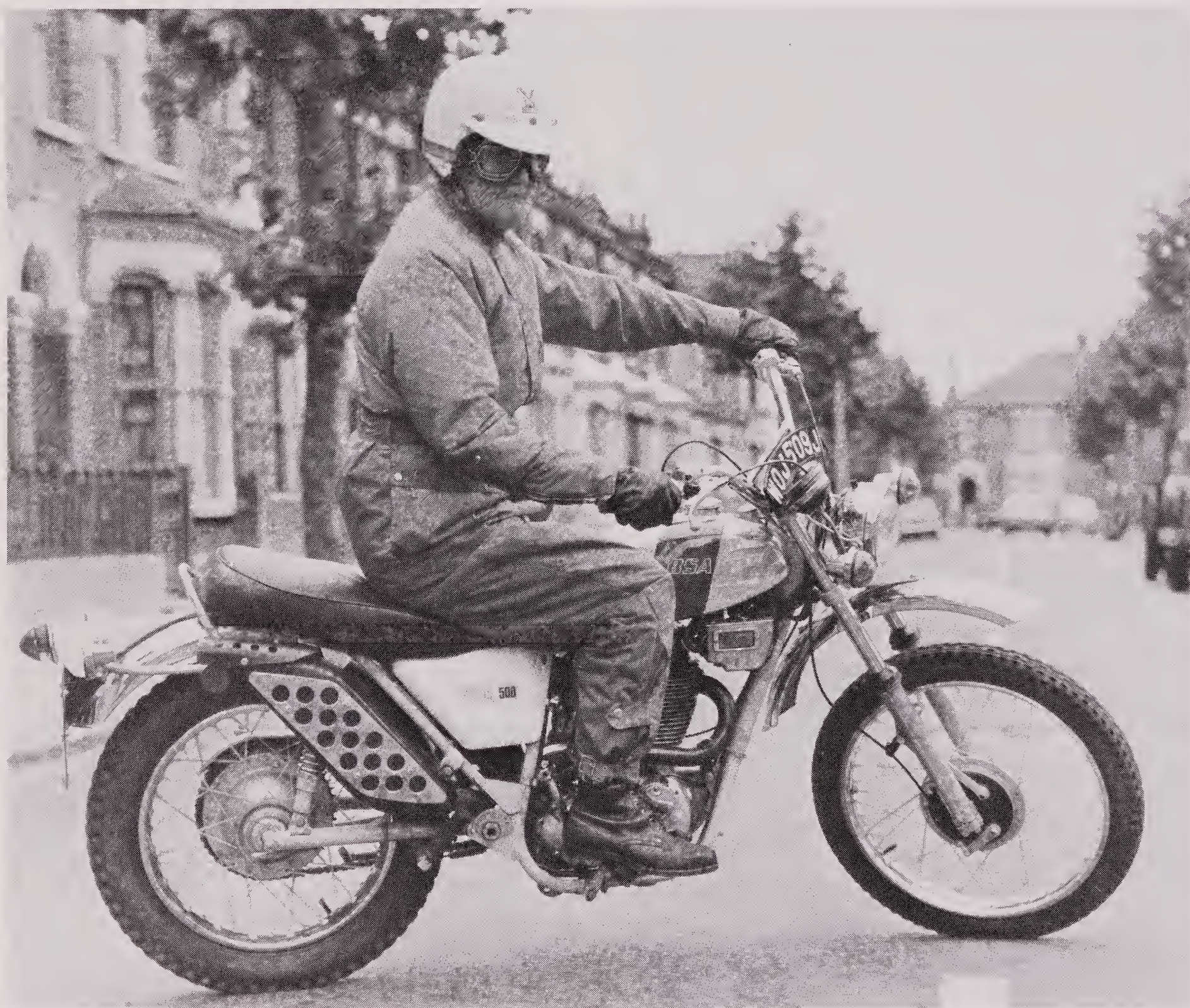
The revamped models of 1971 included this B50T Victor Trail, much as the road machine other than the front mudguard, brake and bars.
