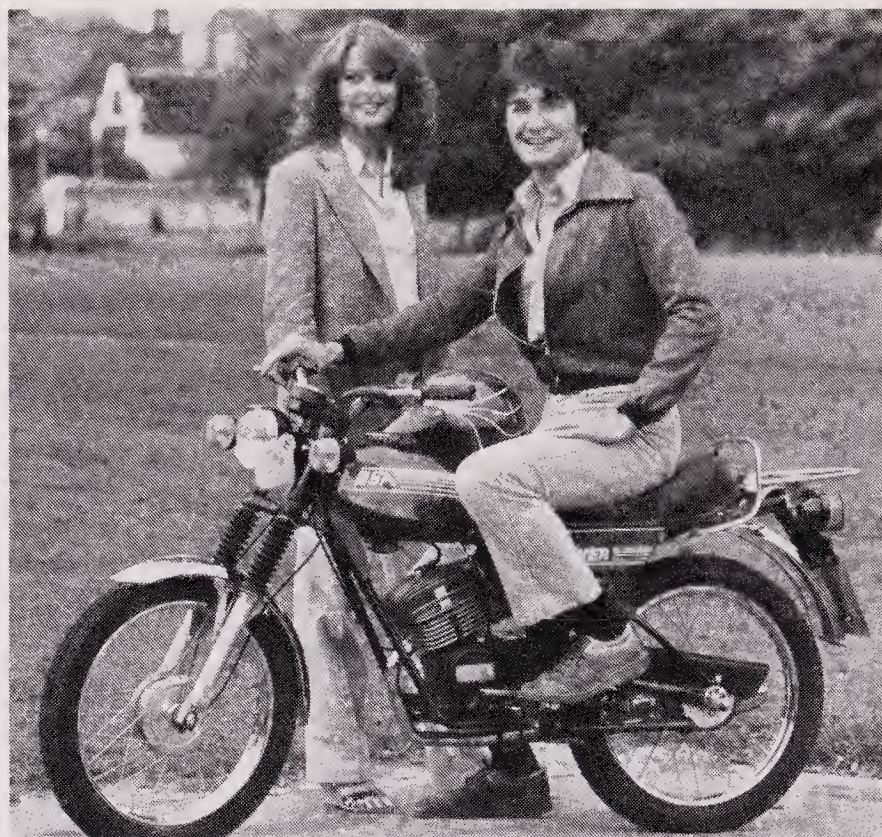
BSA Beaver restricted moped of 1979 with its imported engine. The monoshock rear suspension worked well enough at the speeds the machine could reach.
