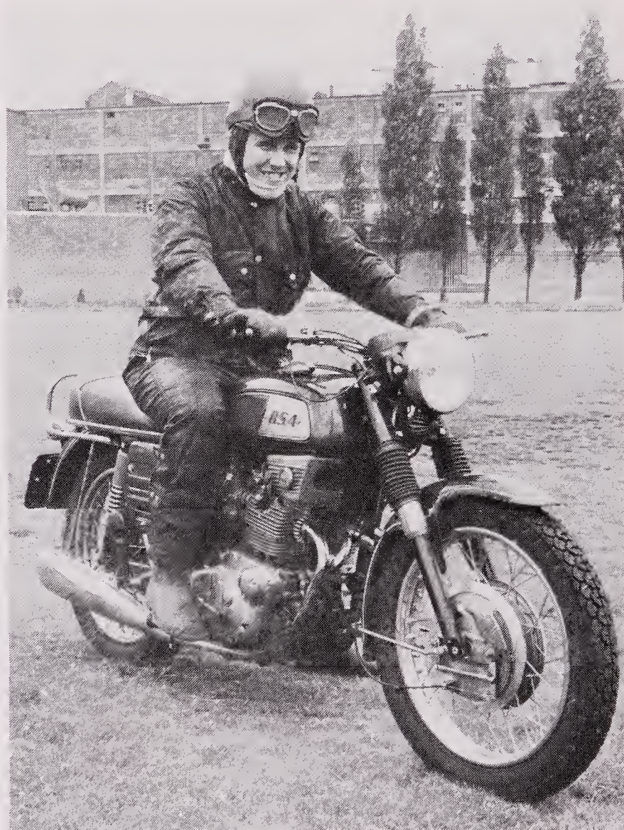
Rocket 3 in its original 1968 form with early type twin leading shoe front brake, here carrying a works tester and with the factory in the background.
