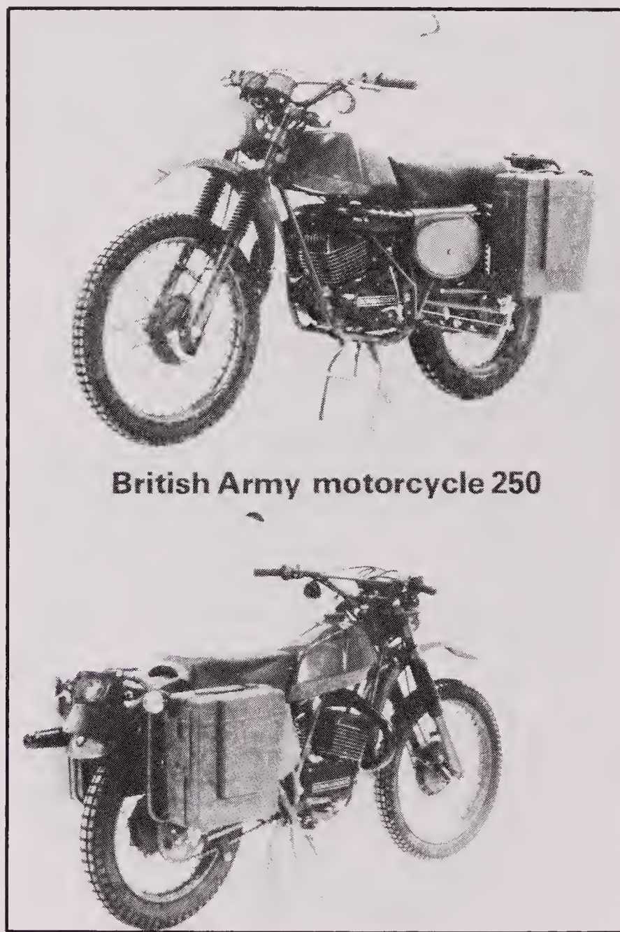
The BSA version of the Canadian Bombardier with Austrian Rotax engine unit as assembled in the British plant in 1979 with a number of UK sourced components.
