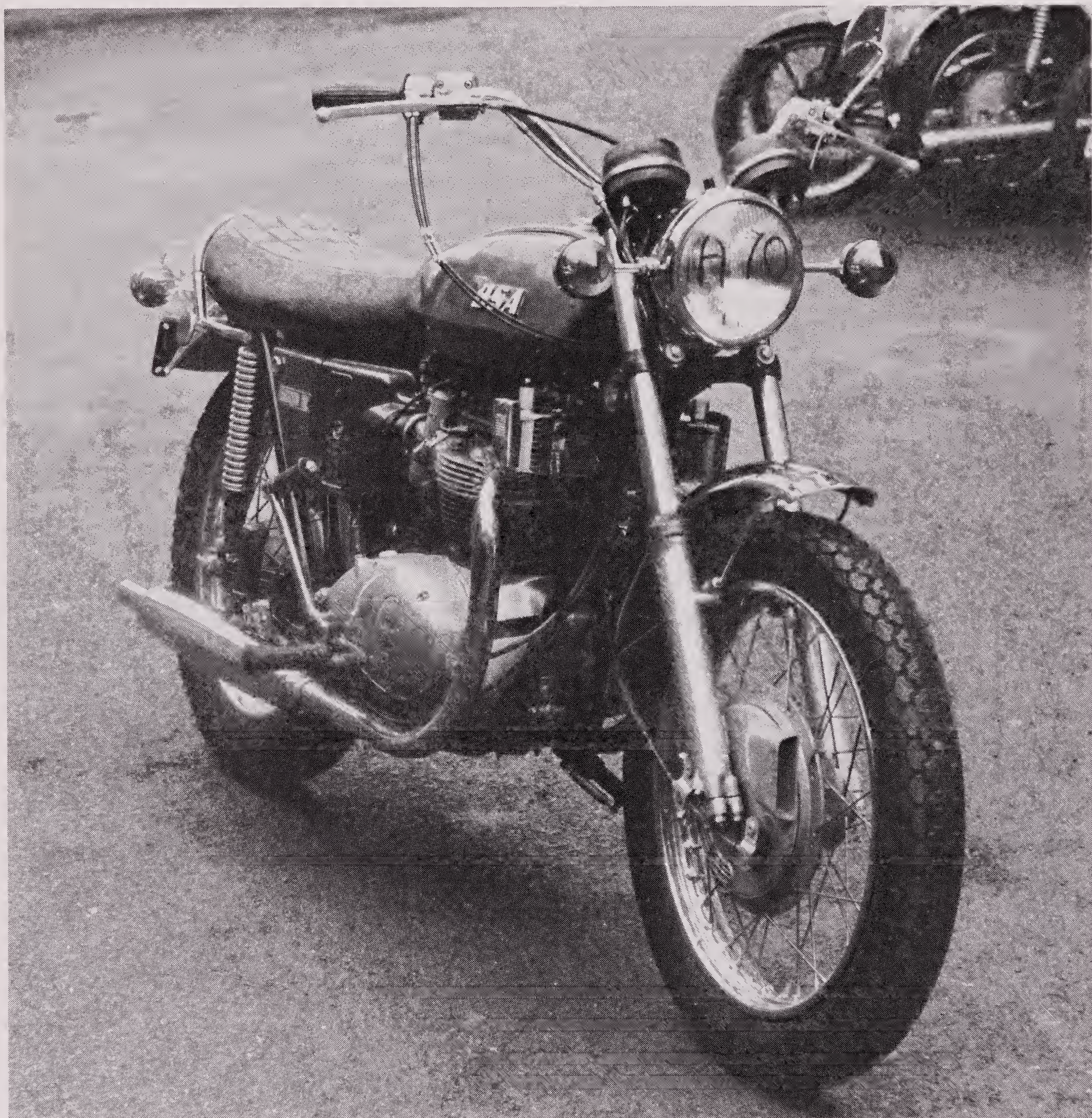
The rare A70L built for the USA but here seen in later years back in its home country. It used the stock cycle parts including the poor front brake.
