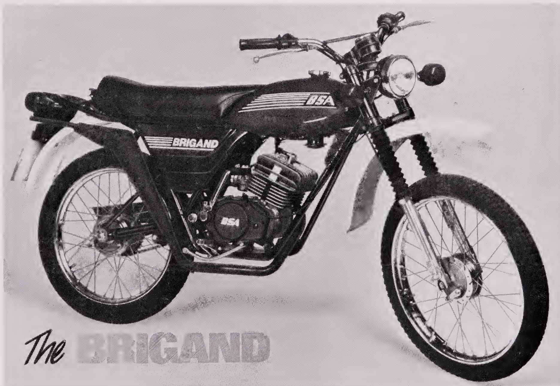
Brigand off-road moped with the Beaver engine and frame, but raised matt black exhaust sys-
