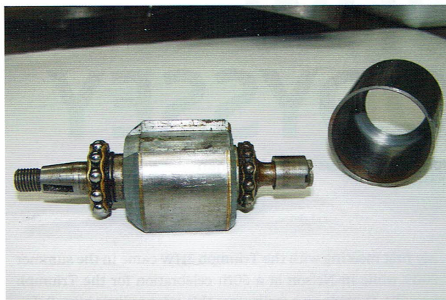
▲ Lucas SR1 rotating magnet (with keeper sleeve)
