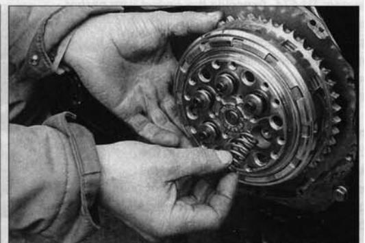
**8** No adjustment of the socket-head set screws is needed on Suzuki clutch. Don't overtighten them into aluminium bosses
