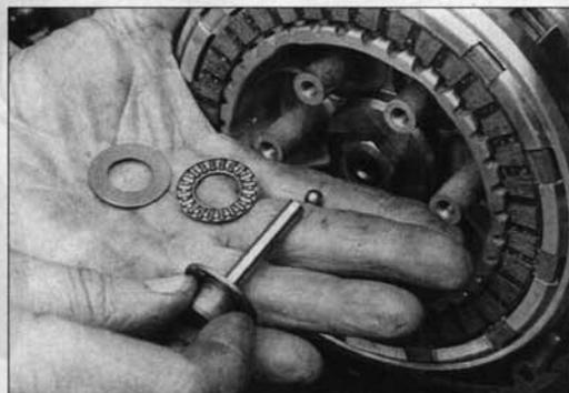
**7** Suzuki top hat and roller thrust race is used with a ball bearing and pushrod. Machined ring on the basket is cosmetic
