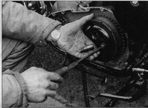
**1** Drain the chaincase, remove its cover, the brake pedal and footrest, split the primary chain and you're ready to tackle the clutch
