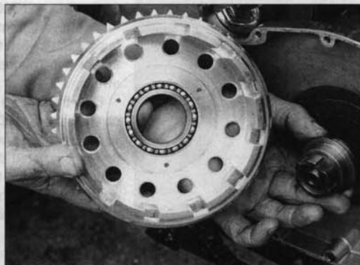
**5** Either seal can be used with Suzuki item which is supplied with an adaptor spigot with or without an oil return scroll
