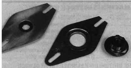
The primary casing becomes oil tight with the oil seal conversion fitted, shown left. It comes with a large cut off splined adapter and costs £48
