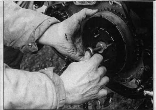
**2** Lock shaft for nut removal by engaging gear and holding down foot brake. Then use a puller (pictured) to withdraw clutch
