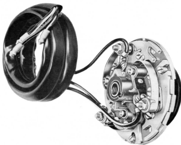
Fig. 29 Contact breaker model 7CA
