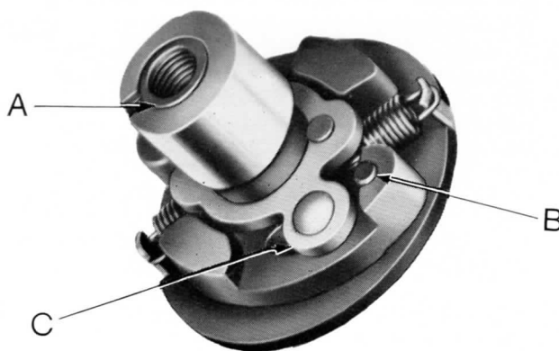
Fig. 30 Auto advance unit used with 6 and 7CA contact breakers
