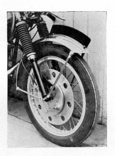
Norwell Alloy Brake Muff. Precision machined from  $\frac{1}{2}$ " Dural 15" diameter. Periphery tapered to  $\frac{1}{8}$ ". Shrunk on to B.S.A. 8" hub after removal of outer fins. Prevents flexing and distortion of hub. Dissipates heat rapidly, minimising brake fade. Can be fitted to new machine or to own wheel. Delivery 10-14 days. Price including fitting. ... £8 10 0
