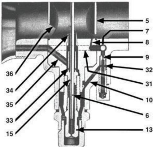
Fig. 3 - Diagrammatic section of Carburettor showing only the lower half of the throttle chamber with the throttle a little open - and the internal primary air passages to the main jet and pilot system
