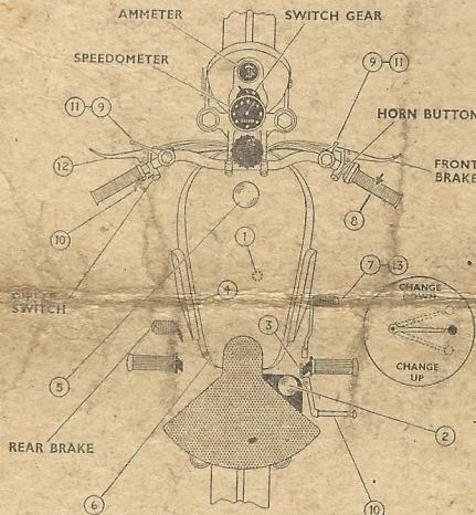
NOTE. To stop with engine running, close throttle, raise clutch lever and apply brakes. To stop engine, close throttle and raise valve lifter.
