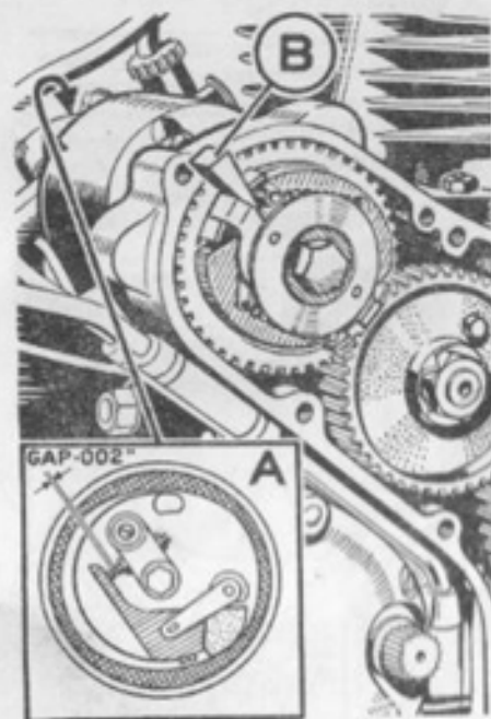
Fig. 7 Automatic Advance (A7 Standard, A10 Golden Flash)
