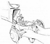
FIG. D2. Removing axle beam.
