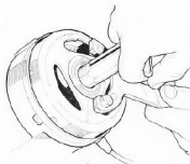
FIG. B11. Releasing flywheel nut.
