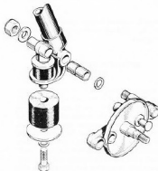
FIG. E4. Front fork exploded.
